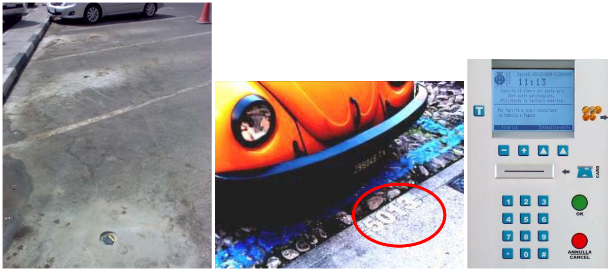
Figure 1: Sensor, parking bay number and parking meters of the TREVISOSTA system.
